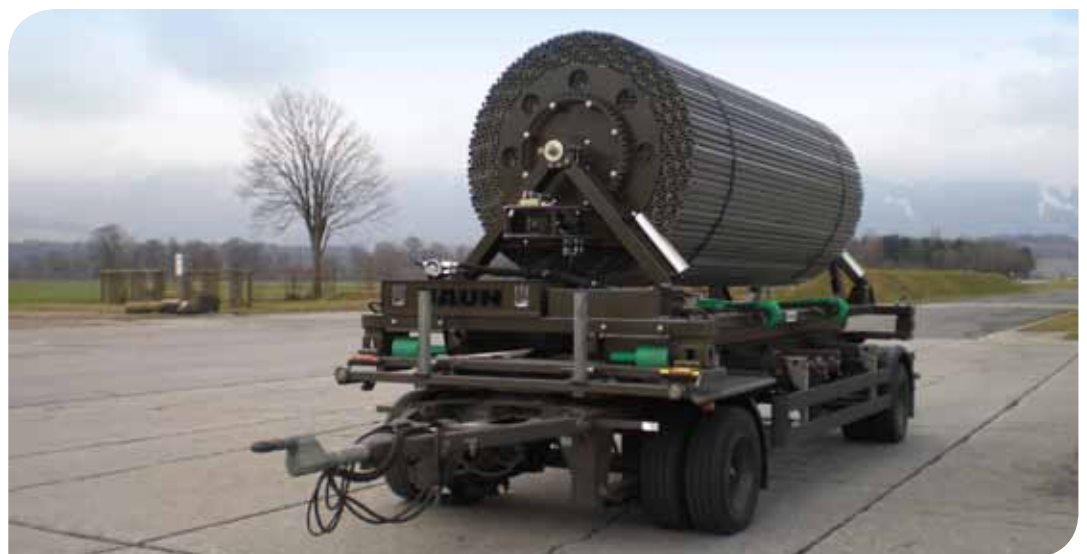
Fig 11: SPOOLRACK, SPOOL ASSEMBLY and TRACKWAY mounted onto trailer
