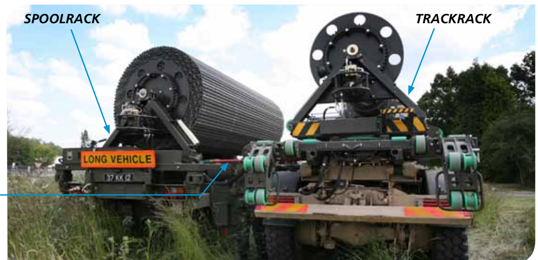
Fig 10: SIGHTING RODS IN USE TO ENSURE CORRECT ALIGNMENT BETWEEN TRACKRACK AND SPOOLRACK
