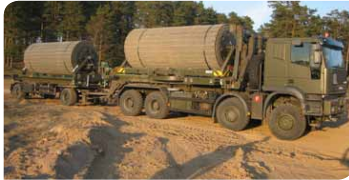
Fig 4: HGMS WITH TRAILER MOUNTED SPOOLRACK
