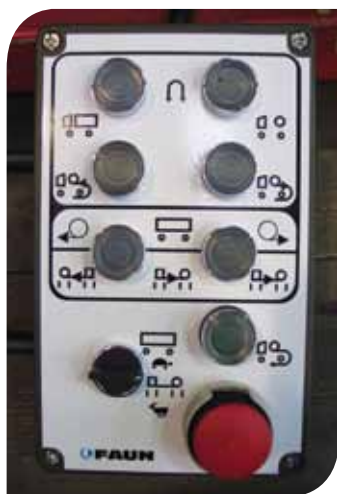
Fig 8: TRACKRACK/ SPOOLRACK CONTROL PENDANT
