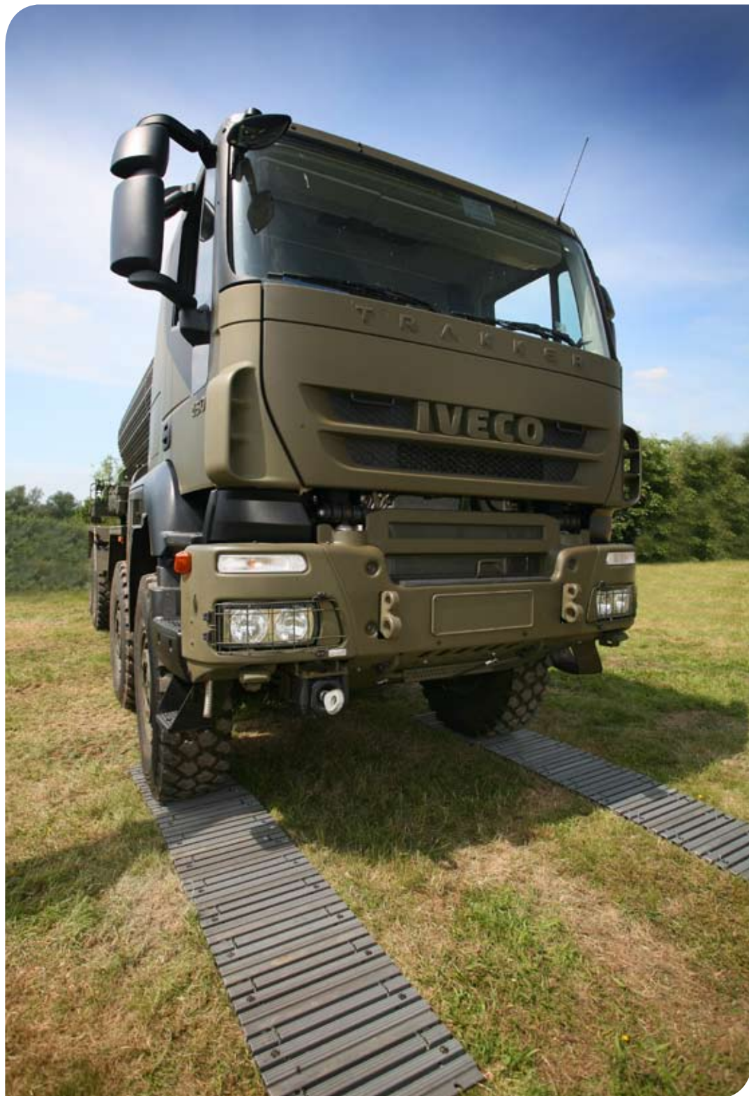
Image 1: IVECO TRAKKER 8x8 on VEHICLE RECOVERY MATS
