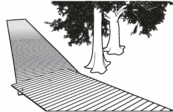
Fig 5-2. Alignment Change to Avoid Natural Obstacle
