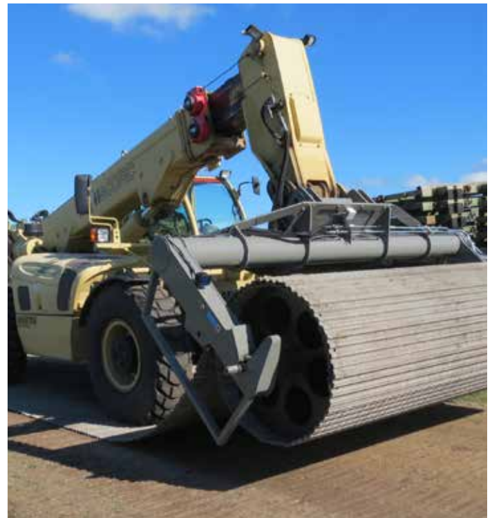
M150 Dispenser (4.2m width) with 40m M150 Trackway® spooled
